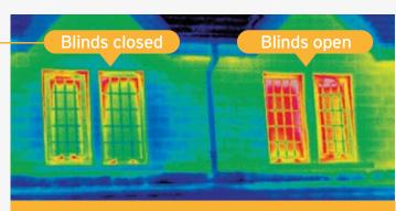
The flow of heat transfer through windows is displayed using infrared imaging. Red areas indicate the highest rate of heat loss.
